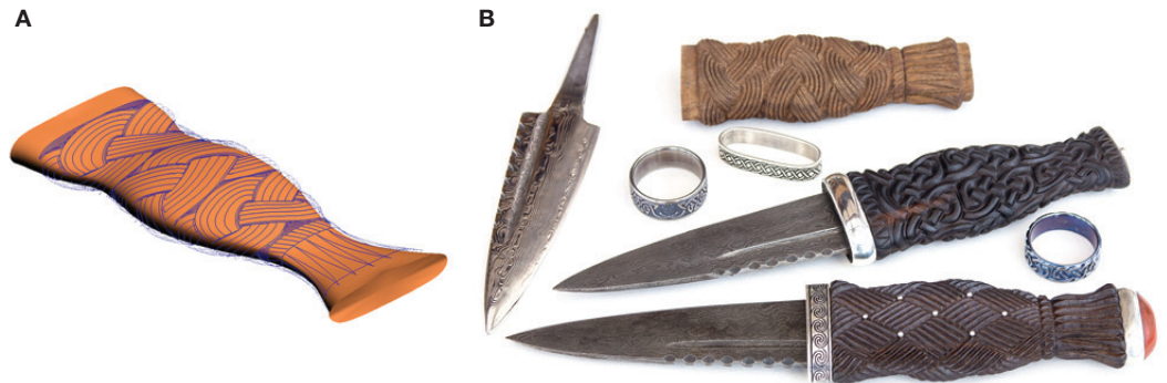
Figure 4. [A] Knife handle milling toolpath generated by Rab Gordon's CNC Toolkit and [B] his celtic knives and jewelry. Photos © 2015 Rab Gordon.
