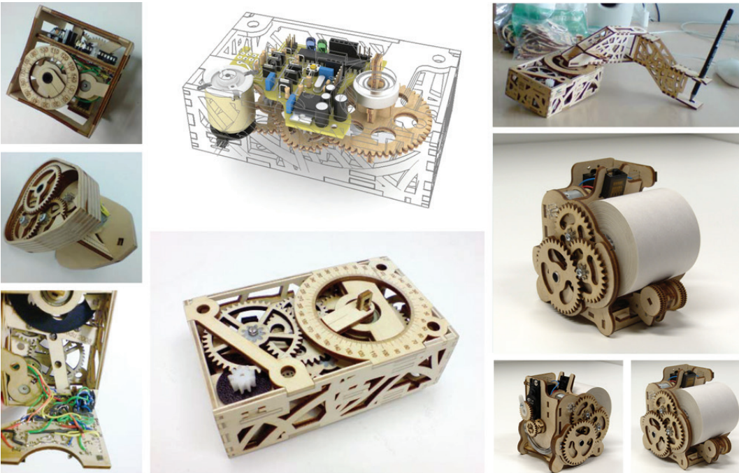
Figure 12. Selections of digitally and manually fabricated plywood machines by Peter Schmitt, using CAD, CNC machine tools, plywood, plastic, metal, electronics and mechanics. Photos © 2006-2010 Peter Schmitt.
