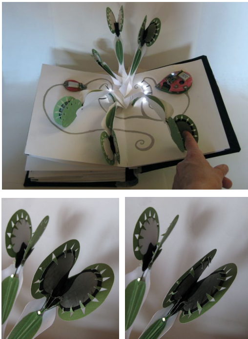
Figure 13. Capacitive sensors trigger nitinol-driven flytraps. Top: a user touches a sensor. Bottom: a trap in its open and contracted states.
