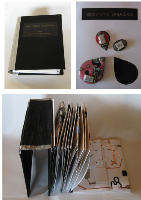
Figure 3. Top, left: the book, right: magnetic electronic modules stored on the first page. Bottom: the book, turned inside-out, showing circuitry on the back of the pages.
