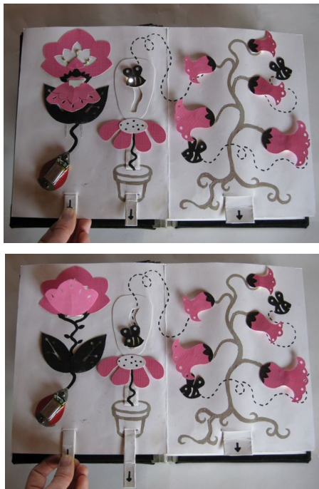
Figure 4. Top: the flower on the left is open and the bee is at the top of its track. Bottom: after pulling the tabs, the flower is closed and the bee is at the bottom of its track, its light turned off. The battery is the dark pink teardrop shape in the lower left hand corner of the page.
